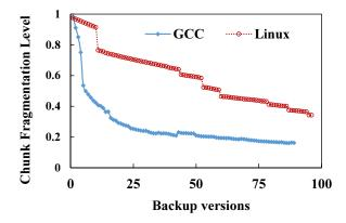
Fig. 1. The chunk fragmentation over time.
