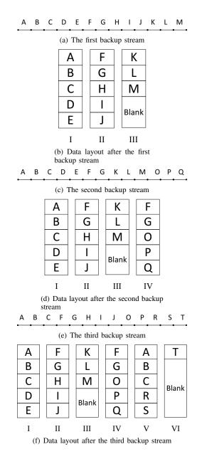
Fig. 3. An example of three consecutive backups with the Capping rewriting scheme.
