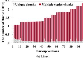
Fig. 4. The redundancy among containers in consecutive versions backups with the Capping rewriting scheme.
