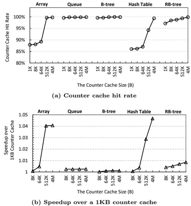
Figure 17: The counter cache hit rates and the performance of SuperMem with different counter cache sizes.
