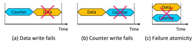
**Figure 4: Different cases when system failures occur.**
