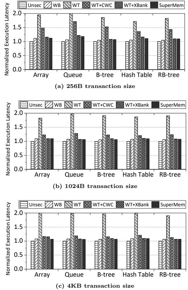
**Figure 13: The average latency of executing transaction requests with different transaction sizes normalized to those of an un-encrypted NVM.**
