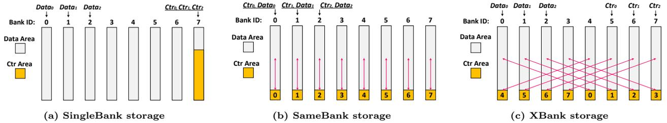
**Figure 8: Different counter storage approaches.** (The number on a counter (*Ctr*) area indicates the bank number storing its corresponding data, e.g., in Figure 8c, the *Ctr* area with the number 4 in Bank 0 stores the counters of data in Bank 4.)
