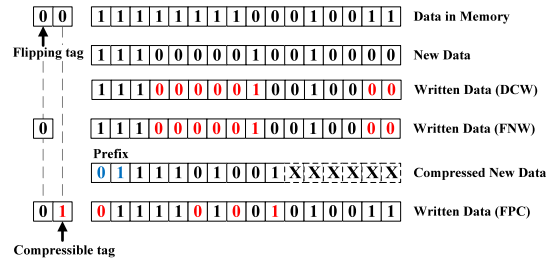
Fig. 2. Illustration of different 16-bit write operations. The data bits in red color need to be written. The blue data bits signify the matching prefix.
